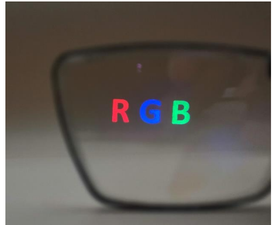
Image 3. Polychrome MicroLED optical module using JBD R, G & B panels, X-cube & Vuzix Polychrome waveguide
