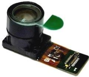
Image 2. MicroLED Projector developed by Vuzix using JBD's 0.13" J013X01VGA microLED display
